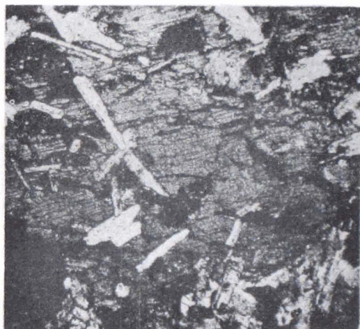
84 Pigeonite with idiomorphic Andesine laths, from Syeno-Diorite, Amlang-La. The Pigeonite is dark, the Andesine clear (G), Ni \times , slice 198. Enlargement 50 times.
