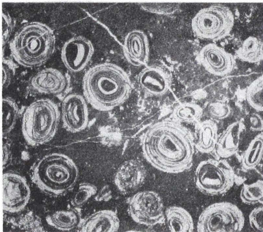
77 Ferruginous Oolite, Callovian, from Laptal. In the dense, impure calcareous matrix are calcite ovoides with varied, partly fragmentary cores (H), slice 251, Enlargement 20 times.
