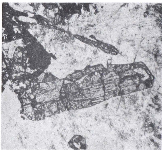
83 Pigeonite of Syeno-Diorite, Amlang-La, Tibet (G), Ni //, slice 200. Pigeonite inside of Perthite. Enlargement 35 times.
